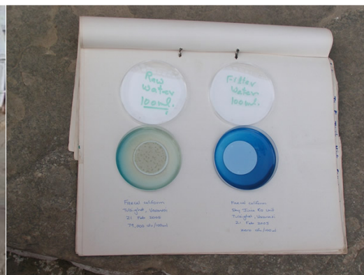
Water filtration test results showing zero counts in the filtrate
