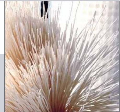
Membrane is a homogeneous PvdF hollow fibre
